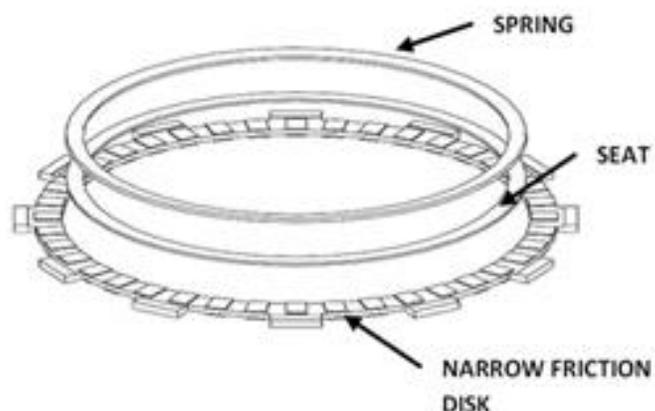
If judder spring and seat are installed, assemble the clutch in the following order.
