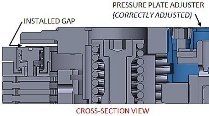
10. Insert the **long end** of a 5-mm hex key into one of the two hex holes in the pressure plate adjuster. By hand, **gently** thread the pressure plate adjuster inward until it comes to a stop against the center clutch nut.
