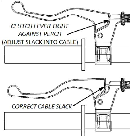
**NOTE:** The pressure plate adjuster should bottom out and lift against the center clutch nut, not the throw-out. Slack in the clutch cable ensures that you find the correct starting point.
