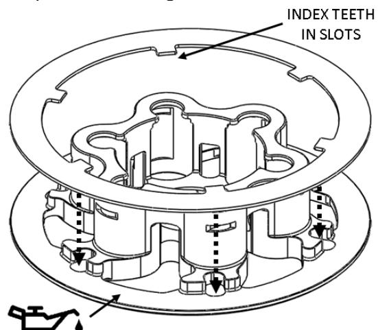
8. Install this pressure plate subassembly.
