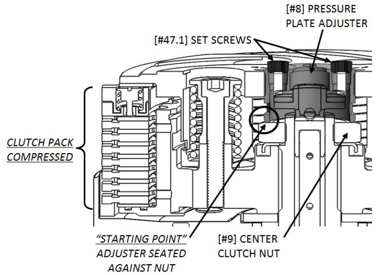
13. Now, insert the **short end** of the 5-mm hex key into the pressure plate adjuster, and turn it clockwise **one full turn plus 2 tick marks past the starting point** (aka “1+2”).
