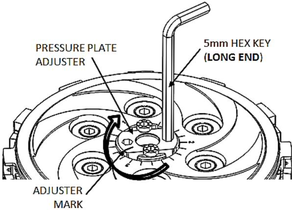
11. At this point, make a note of where the mark on the adjuster aligns with the tick marks on the pressure plate. This is your **starting point**.
