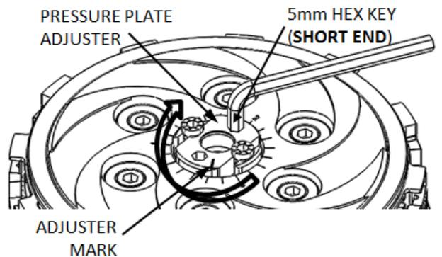
**NOTE:** As you turn the adjuster, the clutch may slip and start to spin before you reach 1-full turn. With the bike in gear you can hold the rear brake for leverage.
